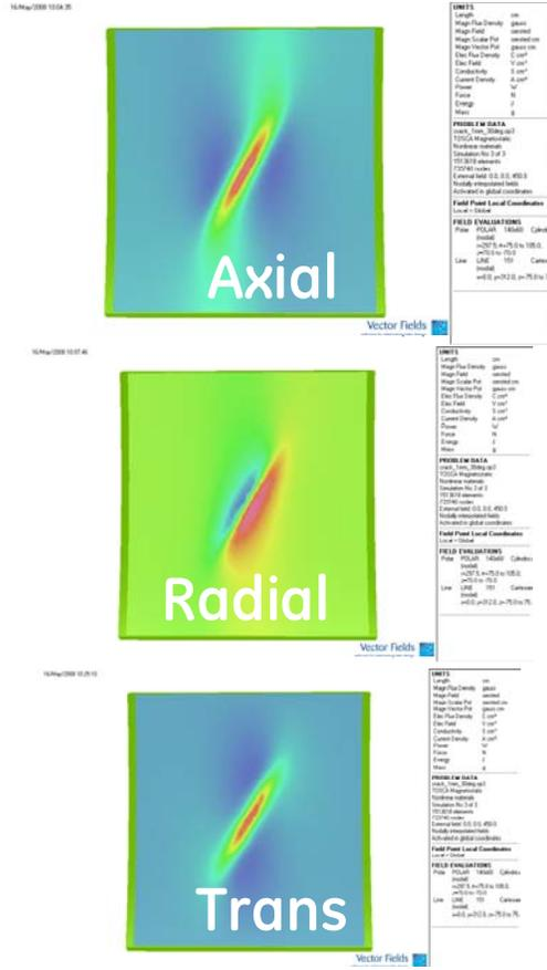
Figure 9. Modeled Crack Magnetic Responses using Finite Element Methods
