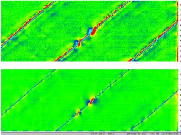
Figure 2 Example of Triax MFL Signal Data with spiral weld distinctly visible
