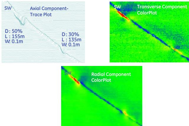
Figure 3. Simulated initial Spiral Weld features via grinding and thin shim plates
